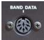
Yaesu FT-1000MP BAND DATA connector
