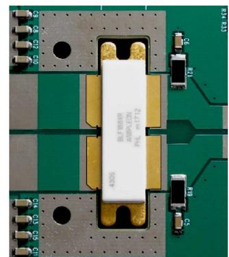
15. Reinstall the copper plates, fold down the Q2 temperature sensor and reinstall the washers and the screws. Pre-tighten all the four screws gradually and check especially that the rectangular washers are properly aligned with the LDMOS. The torque of the LDMOS screws are proper when the spring washers bottom. Tighten the other two screws more tightly.
