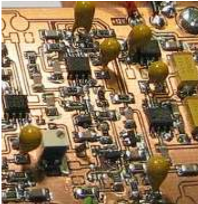
Fig. 11 – Using lead-type tantalum capacitors
