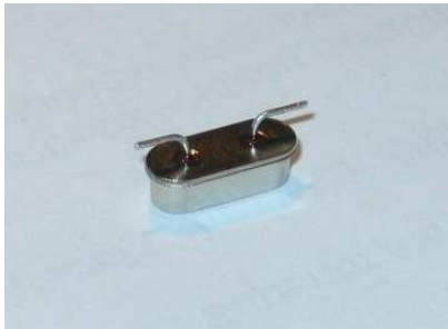
Fig. 7 – Bending crystal "feet"
