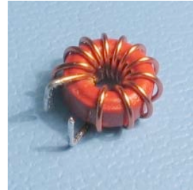
3. Fold the wires for surface soldering
