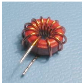
2. Presolder wires with a hot iron
