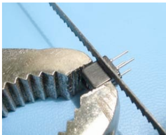
1. Saw or file slots on both sides
