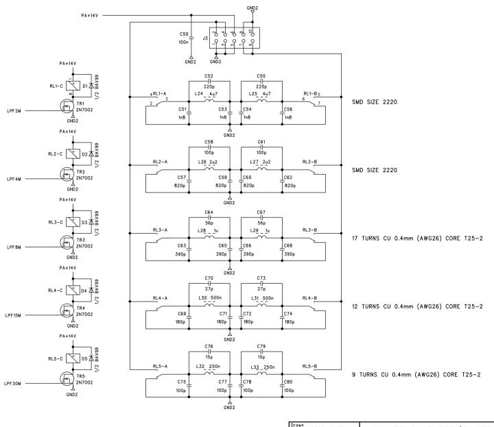
NOTE: Capacitors C52, C55 C58, C61, C64 C67, C70, C73, C76 and C79 are not assembled. They are simulated nulling values for elliptical response.
