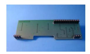
**Function:** The voice memory option is a JUMA TRX2 plug in module which includes audio record and playback functions. It can record from the microphone or from the receiver. Playback can be sent to the band or to the local speaker.
