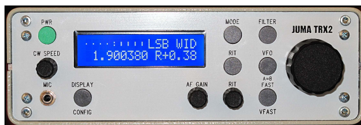
Frequency Display Including RIT Offset
