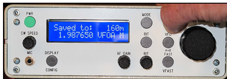
Saving A Frequency To A User Band
